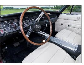
Equipment and options on this striking automobile include the Inland-shifted 4-speed, 3.54 Dana, buckets, console, power steering and brakes, "wood" wheel, and the dealer-installed AM/FM.
