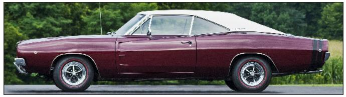
Because the Charger was not ordered with disc brakes, the Ferraras couldn't get 15-inch wheels and had to make do with 14s.
